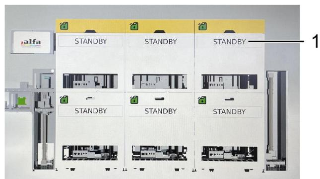
When the machine is switched on, the system runs a reset routine and sets all dispensing heads to STANDBY.
