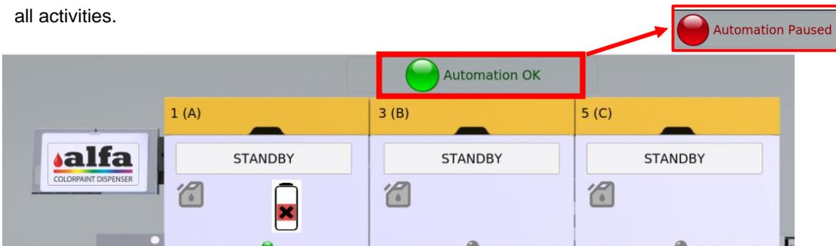
2. When the activities of all dispensing heads are paused, the refill tanks will become green on all dispensing heads. To proceed, please click on the green tank of the dispensing head where the canister to be refilled is positioned. A message of input a barcode will appear.
