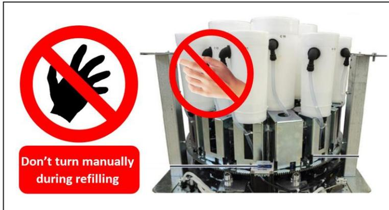
6. When the status switches to DIAGNOSTIC, open the upper cover or the extractable tray. Remove the lid of the canister in the front position. Fill the canister with the appropriate product without exceeding the maximum level (MAX LEVEL).
