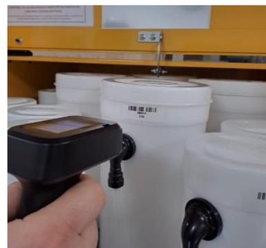
5. If the match is correct, on the screen will appear indication on the circuit, product name, actual fill level and quantity to be refill to achieved the full top level, anyway is possible to chose a different quantity to refill.
