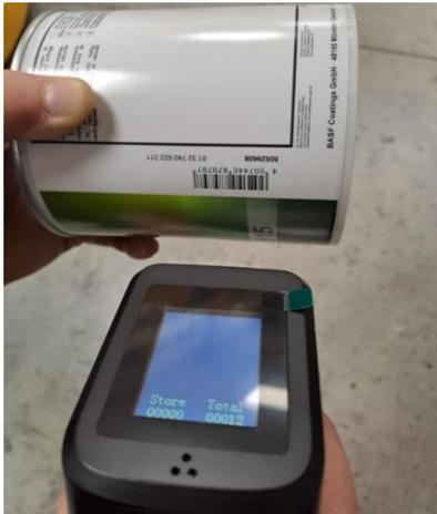
4. The software automatically rotate the carousel by positioning the circuit on the front position of the dispensing head. A message will appear on the screen to verify with the scan the barcode on the canister for a double check.
