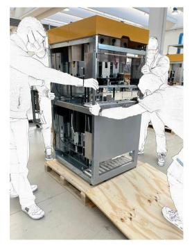
Place the machine in its installation place, on a surface suitable for sustaining its weight or on perfectly smooth and level flooring.
