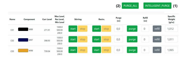
There are also 2 different buttons for the purge cycle: a button to perform the intelligent purge (1) and a button to purge all products (2).
