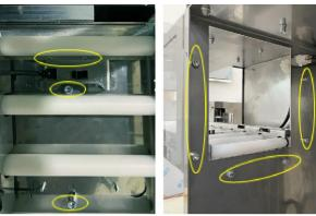
Connect the barcode communication cable (7) and the upper roller conveyor wiring (8).
