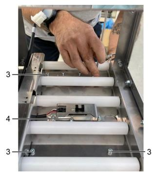
Fit the input roller conveyor over the output tunnel using the 4 M4 TCEI screws with 3mm Allen wrench.
