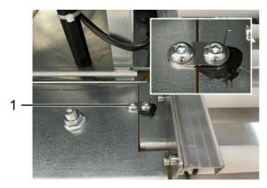
Each turning table is fixed to the fixed part of the cabinet by 3 or 4 stud bolts that prevent its rotation during transport.
