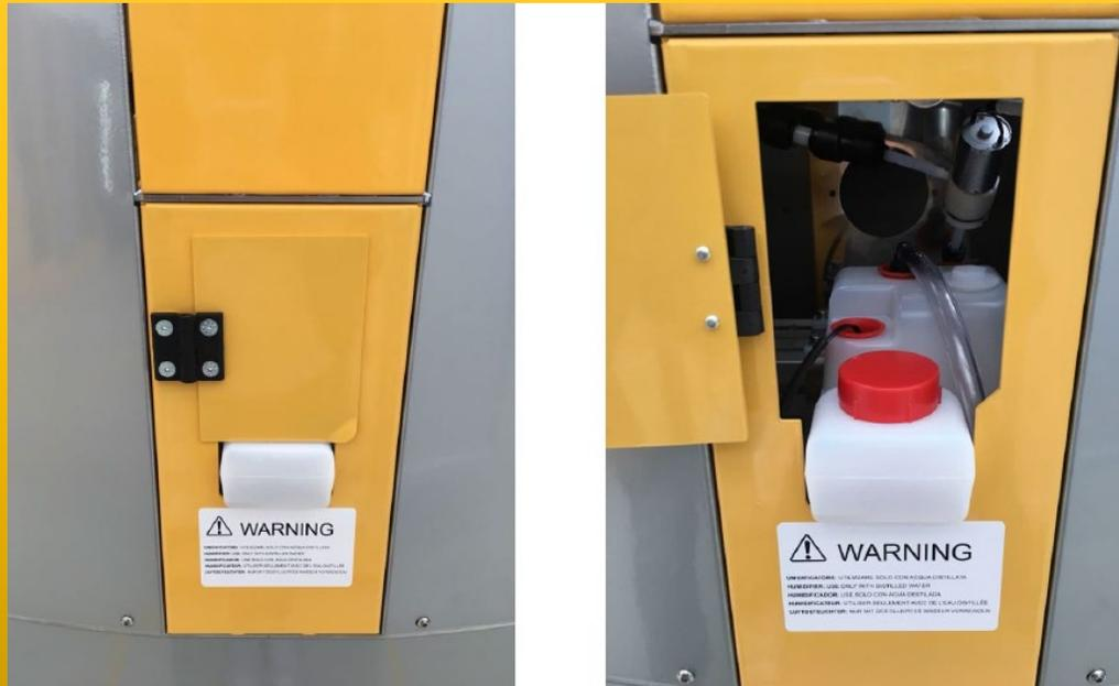
It is located on the left side of the Lab, with an access window for filling the water tank.
