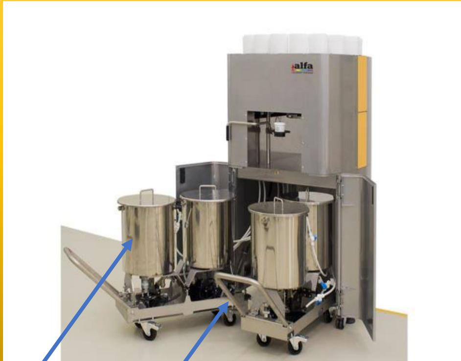
The cabinet can hold 2 trolleys capable of holding up to 4 22-litre stainless steel tanks (1) suitable for holding bases or semi-finished products.
