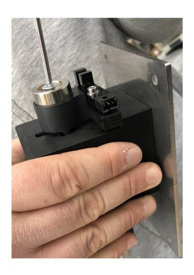
The magnet is fixed on the outside of the mother screw with an allen of m5.
