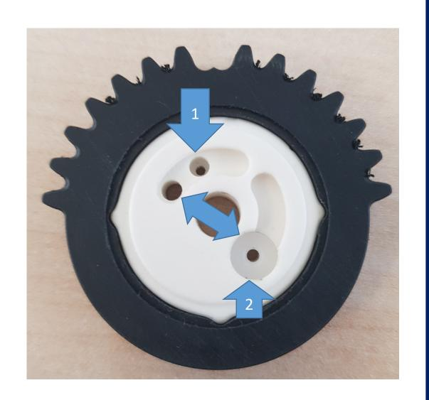
Disc embedded in the gear.
