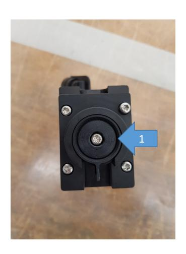
View of the part that is coupled with the motor of the pump, washer (1) of iron that sticks to the magnet that is in the mother screw.
