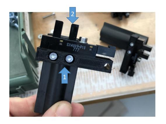
The support (1) of the photocell coupling is fixed on the mother screw with 2 allen 2.5m And the photocell (2) with an allen of 2.5
