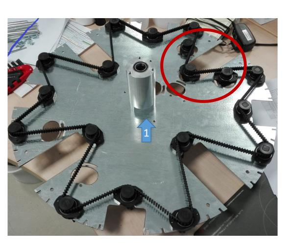
In the lower part of the central sheet we find the belt that makes the agitation couplings move.
