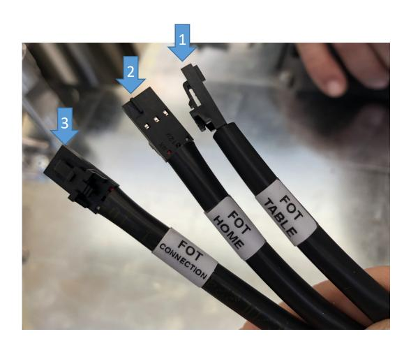
In this image are the three cables for the In this image are the three cables for the photocells.
