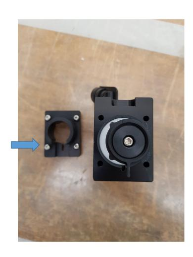
By unscrewing the 4 Torx 4x18 screws, the bellows is accessed
