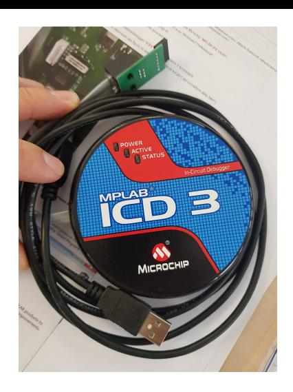
MPLAB ICD 3 programmer.
