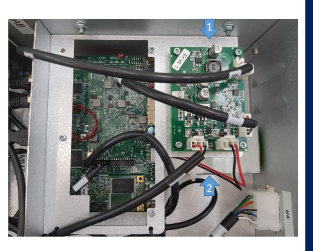
The SPB card (1) fulfills the function of once the machine is turned off to maintain it for about 10 seconds with power to avoid losing the data, the card is powered at 24 volt and with the batteries at 12 (2) volt it feeds the Linux card.
