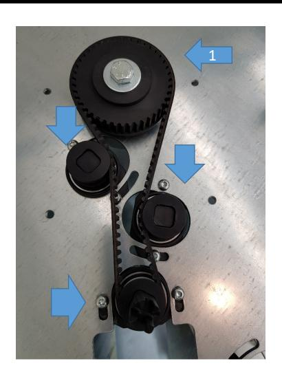
In the central shaft is fixed a gear (1) and a belt that is connected to a stirring coupling, to regulate the tension of the belt the 3 movable tensioners are used.
