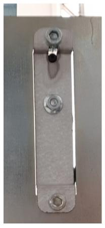
The photocell (1) from the 0 position (home) is fixed to a sheet with an m3 allen, and mounted from the bottom on the chassis with two m4 allen.
