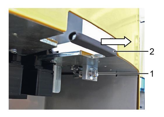
To remove the furniture base trolley it is necessary to unlock the safety stop:
