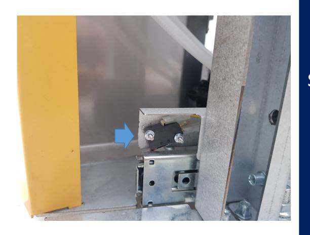
The module of the semifinished has a micro that when it is removed activates and stops all activity, when closing it, a reset must be carried out.
