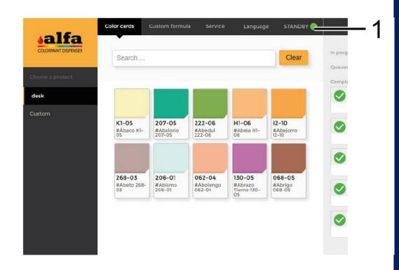
We turn on the equipment and check that it is in (1) green (standby) that there is no alarm.
