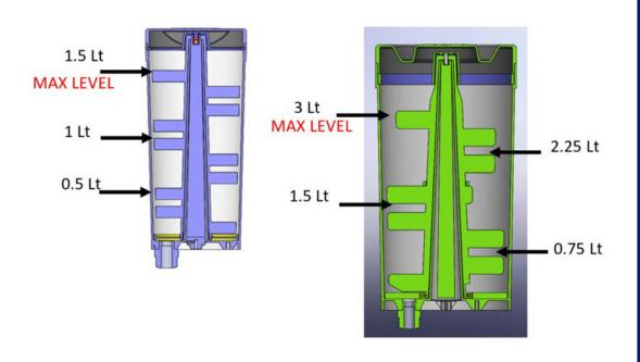
fill the canister with the appropriate pigment until reaching the maximum level indicated (MAX LEVEL).
