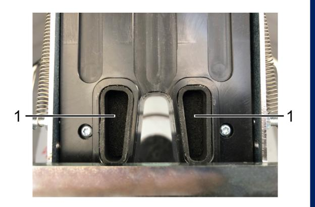
Sponge cleaning Autocap (Thor master) open the Service tab of AlfaTint in DIAGNOSTIC mode (then press the "Open Autocap" button; remove the sponges (1), helping if necessary with a metal thread, and wash them with running water; return the sponges to the original position;
