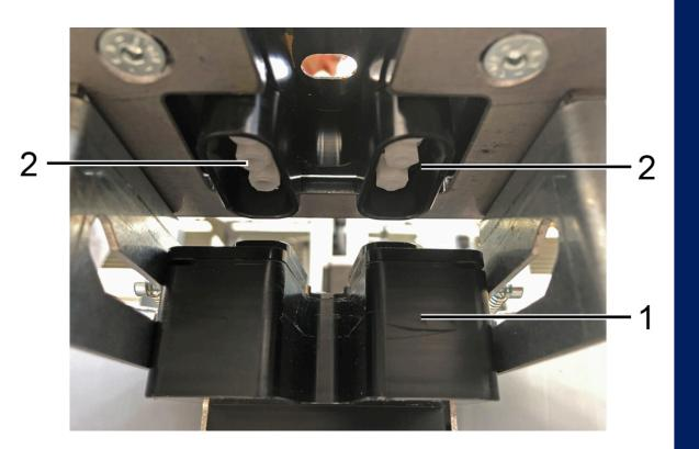
Periodically it is recommended to check that there are no incrustations, deposits or accumulations of dry dye in the injectors.
