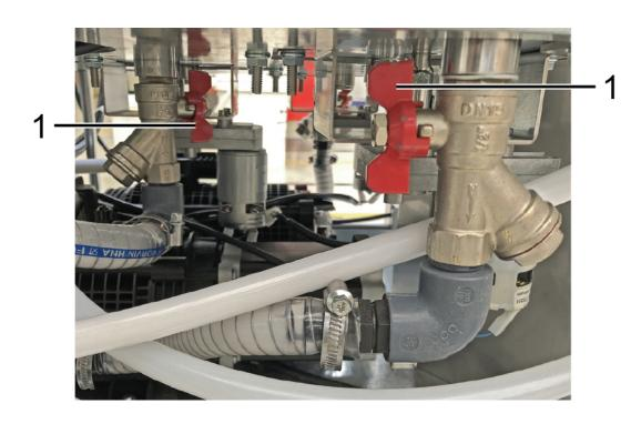
Under the canisters are the respective pumping groups, which are equipped with interception valves (1). At the time of commissioning and before carrying out any tests on the circuits, check that the valves are open.
