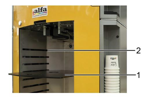
Adjust the height of the platform way the distance between the upper edge of the container that must use and the nozzle is 2-3 cm.
