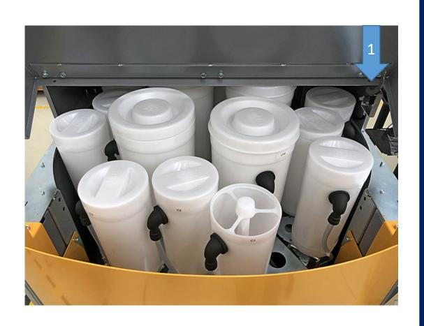
Lifting the lid we have access to the canister to fill them, the lid has a micro (1) that when opened it goes in diagnostic mode, as security so that it does not turn while work is done.
