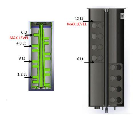
fill the circuits using the corresponding product. Do not fill beyond the level indicated by the terminal part of the stirring paddle (MAX LEVEL).
