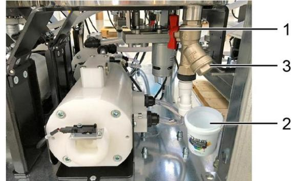
NOTE: A properly positioned can will prevent the product in the filtering compartment from falling and contaminating the surfaces below.
